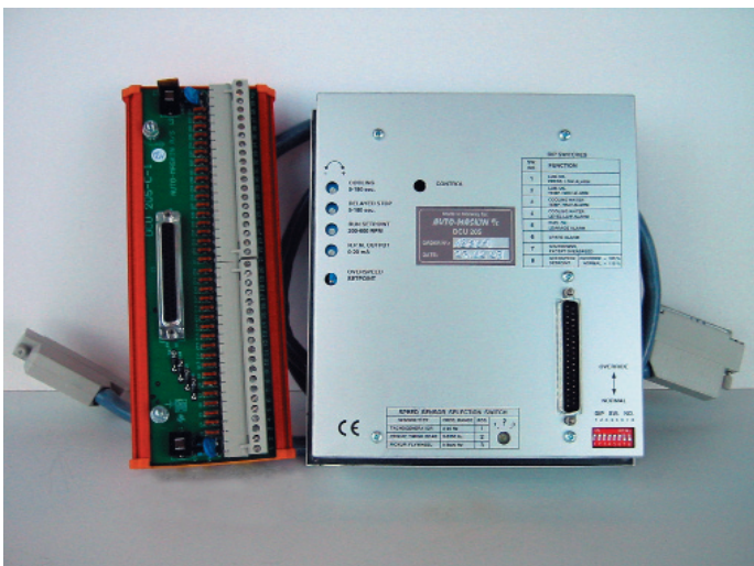
The wire terminal card and the rear side of the control unit. The terminal connectors are "snap" type.
