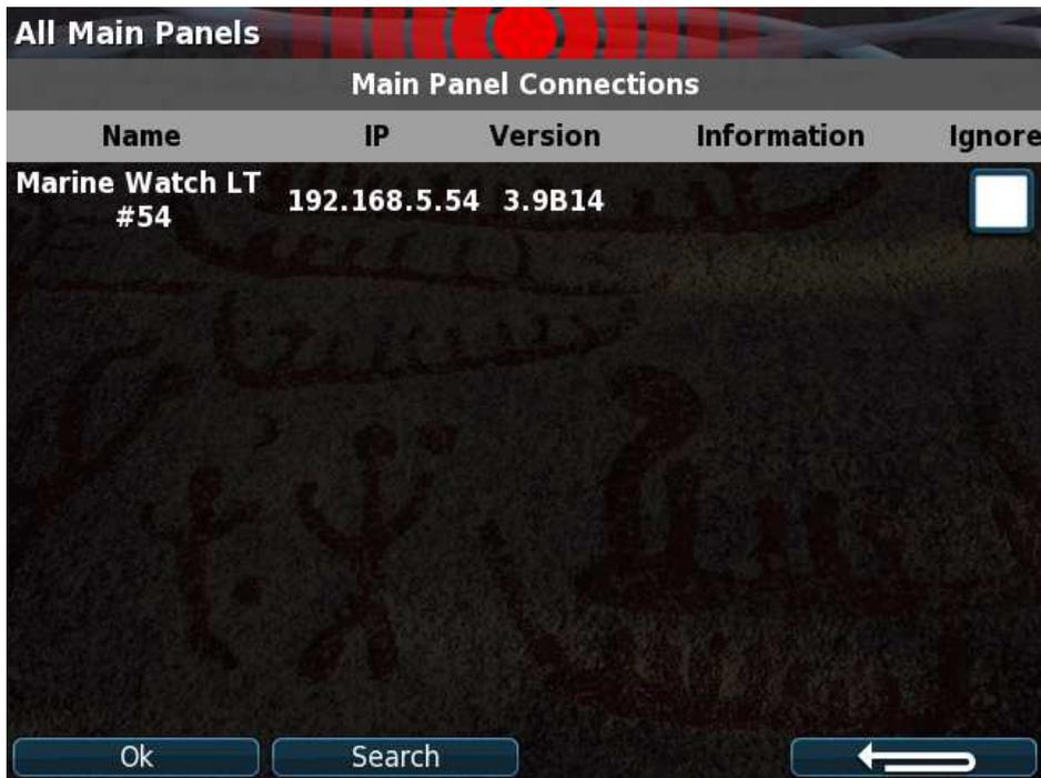
**Note!** The LT-ONE Alarm Panels are identified using the LT-ONE Alarm Panel name and IP address, e.g. “Marine Watch LT #54”, where “Marine Watch LT” is the panel name and #54 are the last digits in the IP address (192.168.1.54).
