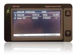
The panel displays a list of up to four engines.
