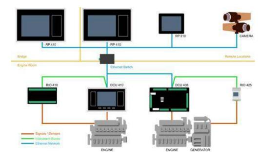
In the one-line diagram example above, multiple panels and equipment is connected together with the switch.
