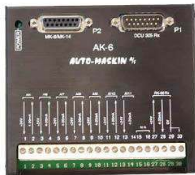
The optional AK-6 analogue card, which adds six 4-20mA channels to the DCU 305 R2.
