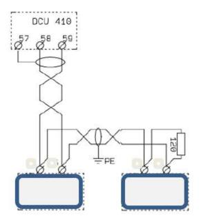
If there are several units attached to the link then connect the 120 ohm resistor together with the last unit on the bus only.
