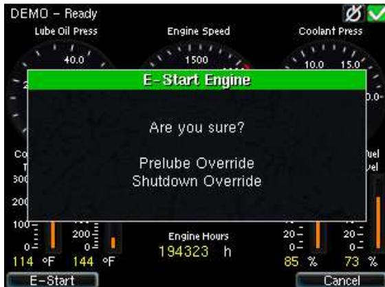
**Note!** Activating E-Start will override any configured Prelube and also set Shutdown Override. The engine will start immediately, and run in a Shutdown Override mode setting.
